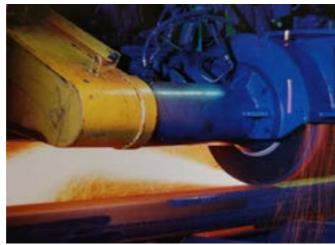
Complete grinding produced perfect surface of billets suitably being supplied for cold heading, cold forging, cold drawing, cold stranding, etc., and other intensive processing works required billets as raw material.
