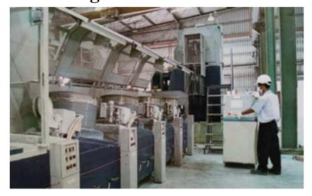
There are four processes for annealed wire production, from intermediate drawing to spheroidized annealing, pickling & coating and skin pass.
